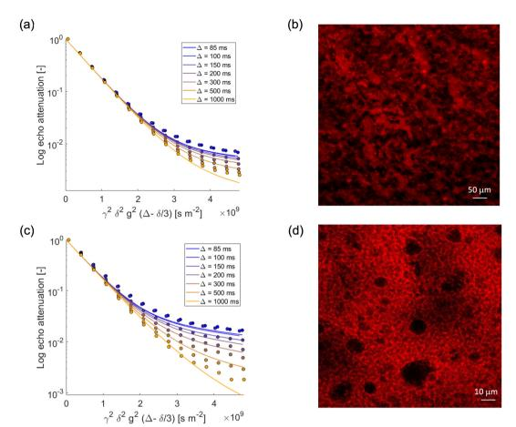
Fig. 4 PGSTE log attenuation plots for (a) water in M/ $G_{1\%}$ , (c) water in M/ $G_{2\%}$  at different observation times  $\Delta = [85, 100, 150, 200, 300, 500, 1000]$  ms. Solid lines are fittings obtained using eqn (2). (b) and (d) Confocal images of  $M/G_{1\%}$ , and  $M/G_{2\%}$ , respectively. Rhodamine B has been used as fluorescent dye.
