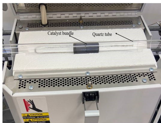
Fig. 1 Quartz tube and catalyst bundle position inside the tube furnace (left), uniformity of the furnace temperature based on data from the manufacturer. 32
