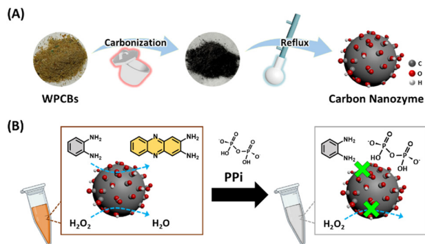
Scheme 1 Schematic illustration of (A) the PPI-responsive CNZ synthesized from WPCBs; (B) PPI induced the peroxidase-mimicking CNZ activity inhibition.
