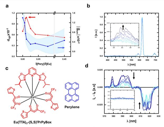
Fig. 5 (a) Plot of  $d_{rgb}$  (red) and  $\tilde{g}_{lum}$  (blue) for a series of PMMA/Eu(TTA)<sub>3</sub>(S,S)- $^{\rm i}$ PrPyBox films containing increasing amounts of perylene. (b) Emission and (d) corresponding CPL spectra of the solution of Eu(TTA)<sub>3</sub>(S,S)- $^{\rm i}$ PrPyBox containing increasing amounts of perylene; the CPL spectra are normalized by the integral of the corresponding total emission spectrum. (c) Eu(TTA)<sub>3</sub>(S,S)- $^{\rm i}$ PrPyBox and perylene.
