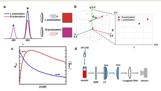
Fig. 1 (a) Illustration of the base principle of CPL photoscopy, with resulting colors under L and R circular polarization. (b) rgb coordinates for the two polarizations on a 3D and a 2D plot. (c) Calculated trend of  $d_{rgb}$  and  $\tilde{g}_{lum}$  as a function of the [A]/[B] emission intensity ratio. (d) Schematic of the experimental setup for the acquisition of the photographs.
