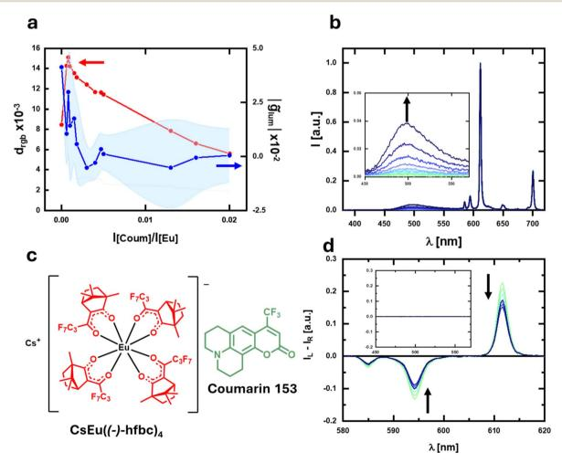
Fig. 4 (a) Plot of  $d_{\text{rgb}}$  (red) and  $\tilde{g}_{\text{lum}}$  (blue) for a solution of CsEu((-)-hfbc)<sub>4</sub> containing increasing amounts of coumarin 153. (b) Emission and (d) corresponding CPL spectra of the solution of CsEu((-)-hfbc)4 containing increasing amounts of coumarin 153; the CPL spectra are normalized by the integral of the corresponding total emission spectrum. (c) CsEu((-)-hfbc)₄ and coumarin 153.
