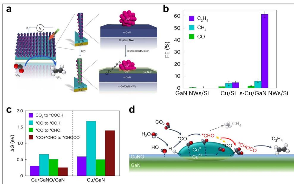
Fig. 17 (a) Schematic diagram of the *in situ* construction of copper clusters and photocathodes. (b) FE of products at different photocathodes. (c) Energy barriers at different steps in the free energy diagram. (d) Possible reaction mechanism of CO<sub>2</sub>RR to C<sub>2</sub>H<sub>4</sub>. Reproduced with permission from ref. 22. Copyright 2024, Springer Nature.
