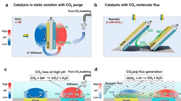
Fig. 8 (a) Schematic diagram and (c) mechanism diagram of the traditional PEC device using static solution. (b) A schematic diagram and (d) mechanism diagram of  $\text{CO}_2$  flux catalysis with clear boundary layer shear flow. Reproduced with permission from ref. 109. Copyright 2025, Springer Nature.
