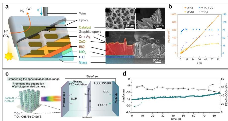
Fig. 19 (a) Schematic depiction of the BiOI photocathode with its components. (b) The stability test. Reproduced with permission from ref. 167. Copyright 2022, Springer Nature. (c) Schematic diagram of solar-driven bias-free PEC-CO<sub>2</sub>RR system for formic acid production. (d) The stability test. Reproduced with permission from ref. 201. Copyright 2025, Wiley-VCH GmbH.
