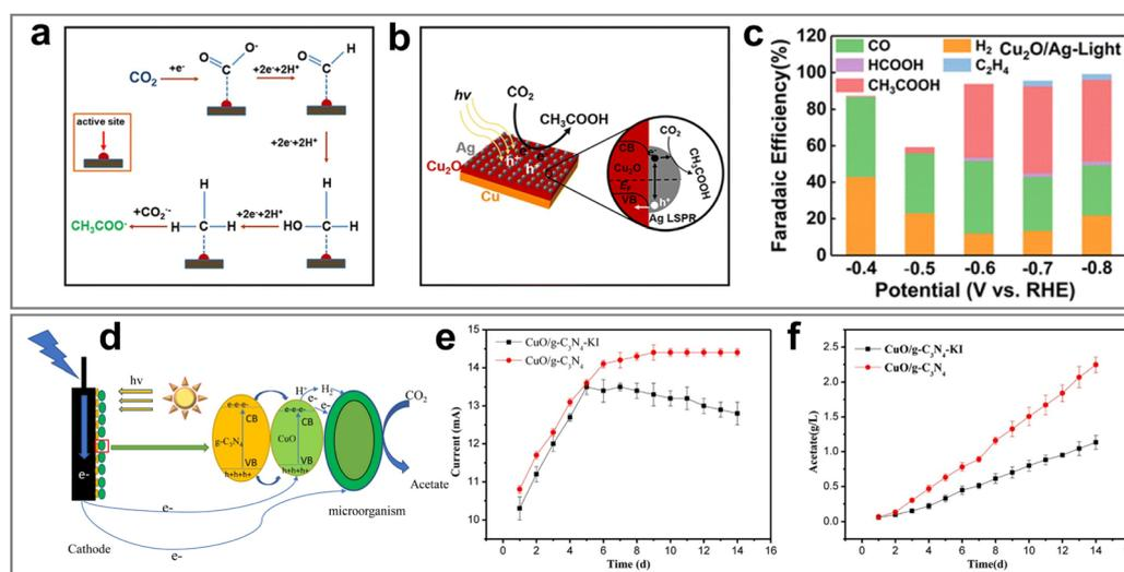
Fig. 16 (a) Schematic diagram of reaction pathways. (b) Charge transport diagram of  $\text{Cu}_2\text{O/Ag}$  for PEC  $\text{CO}_2\text{RR}$ . (c) FE of products on the cathode under different applied potentials. Reproduced with permission from ref. 238. Copyright 2022, The Royal Society of Chemistry (d) Photocatalytic mechanism of MES. Comparison of (e) current density and (f) acetate yield. Reproduced with permission from ref. 242. Copyright 2021, published by Elsevier B.V.
