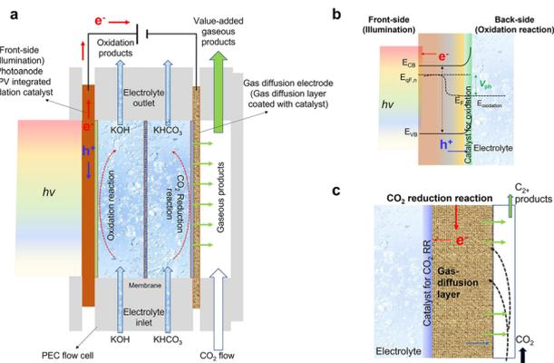
Fig. 5 Schematic of a PEC flow cell for CO<sub>2</sub>RR using a GDE. (a) Schematic of PEC flow cell for CO<sub>2</sub>RR using a photoanode or a PV-integrated oxidation catalyst and a GDE. (b) Requirements of a photoanode/oxidation catalyst. (c) The GDE consists of a CO<sub>2</sub>RR catalyst coated on a porous gas-diffusion layer. Reproduced with permission from ref. 9. Copyright 2023, Elsevier B.V. All rights reserved.
