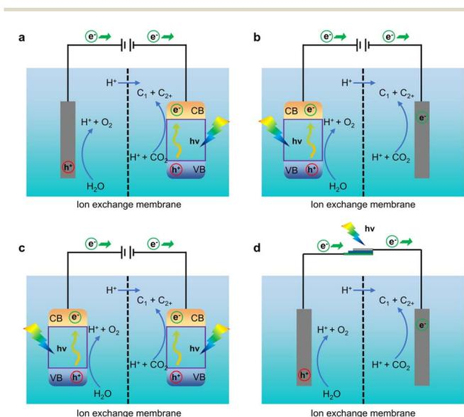
Fig. 4 Device types of photocatalytic  $\text{CO}_2$  reduction systems. (a) The photocathode drive system, (b) the photoanode drive system, (c) the photoanode and photocathode co-drive system, and (d) the hybrid optical system combining the electrode with the photovoltaic cell.
