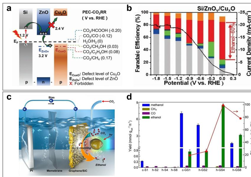
Fig. 18 (a) Schematic illustration of the designed defect nanomaterial structure for selective PEC  $\text{CO}_2\text{RR}$  to ethanol. (b) FE of ethanol. Reproduced with permission from ref. 257. Copyright 2023, Wiley-VCH GmbH (c) Mechanistic demonstration of the PEC  $\text{CO}_2\text{RR}$ . (d) Comparison of PEC  $\text{CO}_2\text{RR}$  properties of different samples. Reproduced with permission from ref. 254. Copyright 2023, Wiley-VCH GmbH.
