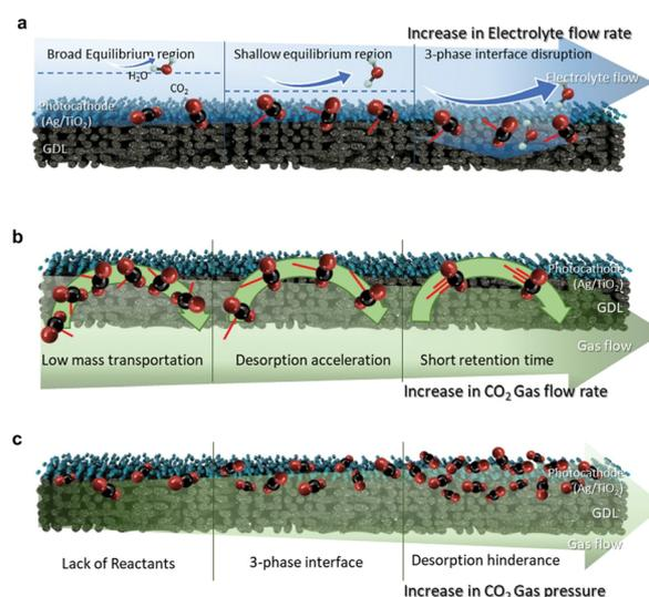
Fig. 9 Diagrams of the surface of the gas diffusion photocathode at different (a) electrolyte flow rates, (b) gas flow rates and (c) gas pressures. Reproduced with permission from ref. 110. Copyright 2024, Wiley-VCH GmbH.
