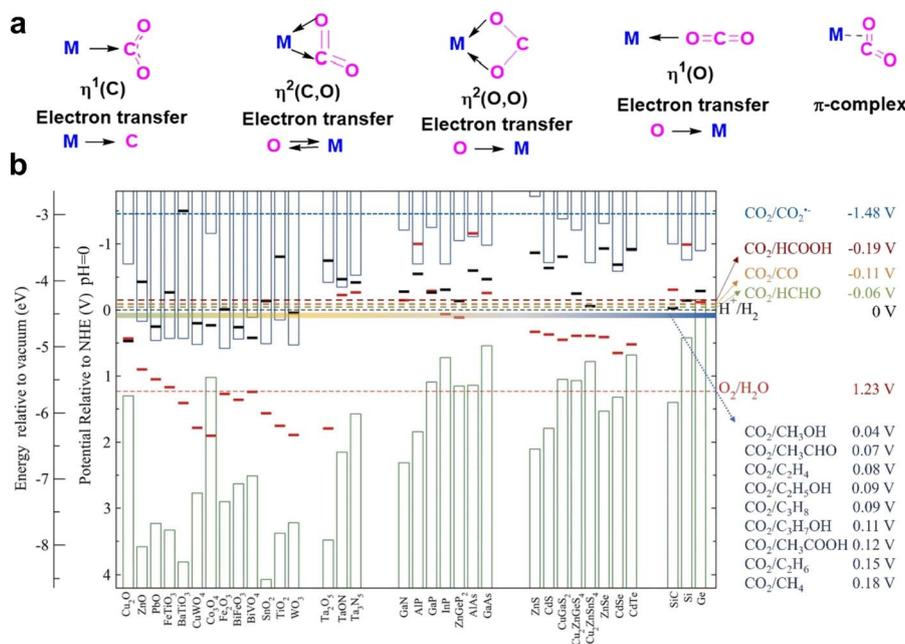
Fig. 10 (a) Common methods of CO<sub>2</sub> activation. Reproduced with permission from ref. 112. Copyright 2023, American Chemical Society. (b) The bias potentials, conduction band positions and valence band positions of various CO<sub>2</sub> reduction reactions, and the calculated semiconductor oxidation and reduction potentials. Reproduced with permission from ref. 115. Copyright 2024, published by Elsevier B.V.
