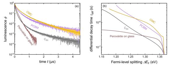
Fig. 15 (a) Tr-PL measurements of three different samples with the layer stack Me-4PACz/triple-cation perovskite/ETL, where the ETL is PCBM, CMC, or  $C_{60}$ . Furthermore, the tr-PL decay of the perovskite film on glass is presented as a reference. (b) Differential decay times were calculated from the fitted tr-PL data as a function of Fermi-level splitting. Figure reproduced from ref. 30 under the terms of the CC-BY 4.0 license. © The authors of ref. 30 (2023).
