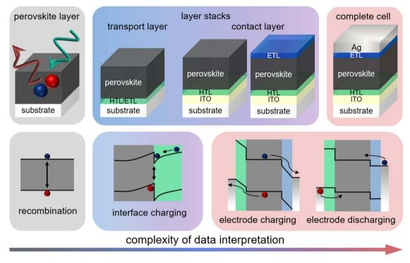
Fig. 9 Upper row: layer stacks from films on a glass substrate *via* films with transport and contact layers, such as ITO, towards complete cells. Bottom row: schematic band diagrams showing the processes that affect transient photoluminescence measurements. Figure reproduced from ref. 33 under the terms of the CC-BY 4.0 license. © The authors of ref. 33 (2021).
