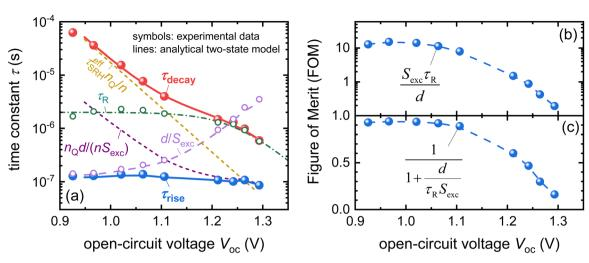
Fig. 17 (a) Time constants extracted from the TPV rise and decay compared with the different terms in eqn (22) and (23) which are shown as dashed or dash-dotted lines. (b) and (c) Figures of merit that follow from the analysis of the rise and decay times shown in panel (a). Reproduced from ref. 17 under the terms of the CC-BY 4.0 license. © The authors of ref. 17 (2023).
