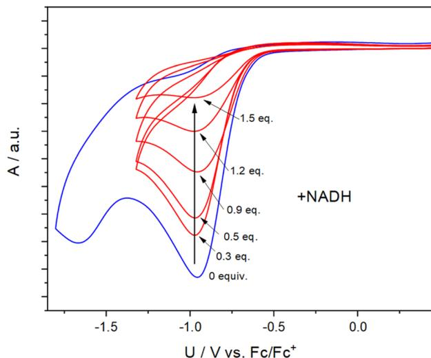
Fig. 3 Cyclic voltammogram of **1c** (blue curve, 30 mM concentration, solvent: MeCN, scan rate: 500 mV s<sup>-1</sup>, supporting salt: Bu<sub>4</sub>NClO<sub>4</sub> (0.1 M), working electrode: Pt). The red curves indicate the decrease of the reduction peak upon addition of NADH.
