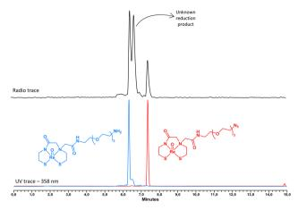
Fig. 5 Radio-HPLC chromatogram of the crude labelling mixture (black) compared to the UV chromatograms of the  $^{\text{nat}}$ Re(v) complexes, Re-4 (red) and  $^{\text{nat}}$ ReO(N<sub>2</sub>S<sub>2</sub>-PEG<sub>3</sub>-NH<sub>2</sub>), produced by the reduction of Re-4 by excess SnCl<sub>2</sub> in ethanol at room temperature (blue).
