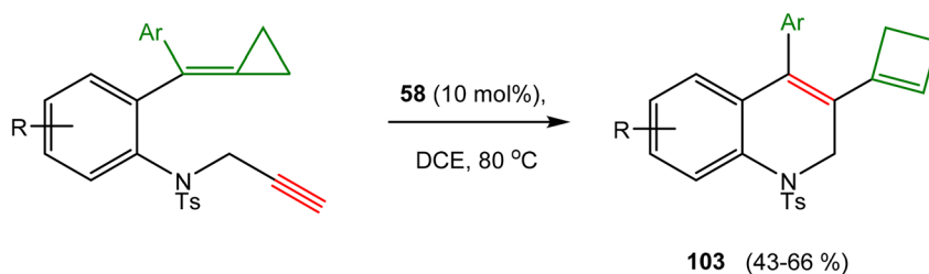
Scheme 41 NHC-gold-catalyzed intramolecular annulation of aniline-linked 1,7-enynes.
