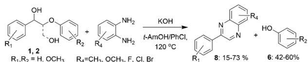
Scheme 4 Conversion of \beta -O-4 lignin model alcohols to quinoxalines.
