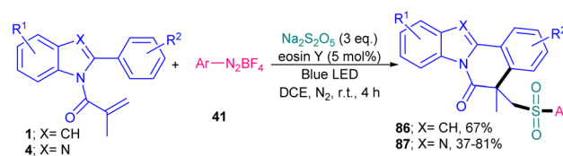
Scheme 40 Eosin Y-catalyzed sulfonylation/cyclization of N -acryloyl 2-aryl indoles/benzimidazoles.
