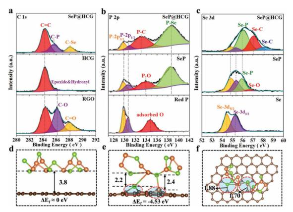
Fig. 5 XPS characterization: (a) C 1s spectrum of HCG, RGO, and SeP@HCG, (b) P 2p spectrum and (c) Se 3d spectrum. And optimized configurations for the adsorption of SeP on various graphene substrates (green sphere for Se, light brown sphere for P, small dark brown sphere for C), (d) side view of perfect graphene (C: Se: P = 60: 8: 8), (e) side view of graphene with two "C" defects (C: Se: P = 58: 8: 8), and (f) planform of graphene with two "C" defects.84
