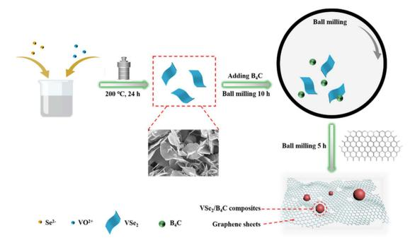
Fig. 3 Schematic preparation of the synthesis of VSe<sub>2</sub>/B<sub>4</sub>C@HCG.<sup>70</sup>
