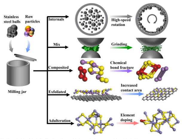
Fig. 1 Working principle of the ball milling jar and potential changes in the raw material particles inside
