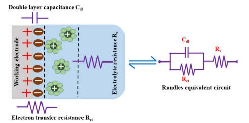
Fig. 13 Charge storage via EDLC formation and the equivalent circuit.
