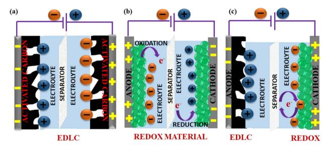
Fig. 10 Schematic of the energy storage mechanisms in SCs: (a) EDLC through surface adsorption/desorption, (b) pseudocapacitance based on the surface redox reaction and (c) hybrid SCs with a combination of non-faradaic and faradaic reactions.
