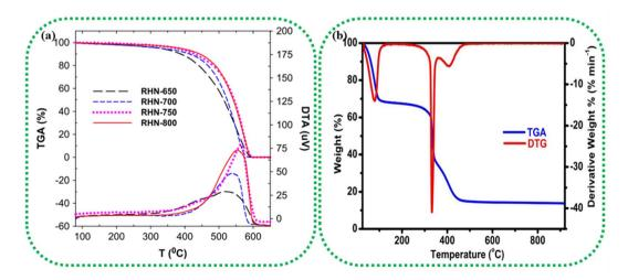
Fig. 2 (a) TGA/DTA analysis of pinewood-derived activated carbon using different activating agents, such as  $H_3PO_4$ , KOH, and  $H_2O_2$ , and heat-only treatments. Reprinted with permission from ref. 93, copyright 2014, Elsevier. (b) TGA/DTG analysis of activated carbon prepared from rice husk at 850 °C under an  $O_2$  atmosphere. Reprinted with permission from ref. 94, copyright 2016, Elsevier.
