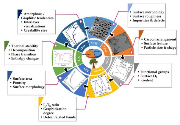
Schematic of multiple techniques used for characterizing BDAC materials.
