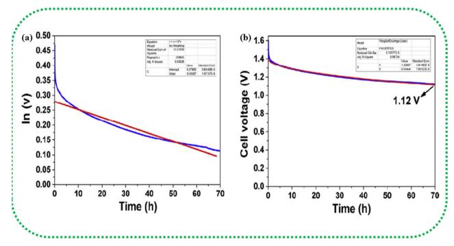
Fig. 15 Curve fitting of the self-discharge model. (a) Leakage current over resistance model (b) diffusion control process model. Reprinted with permission from ref. 212, copyright (2017), Elsevier.
