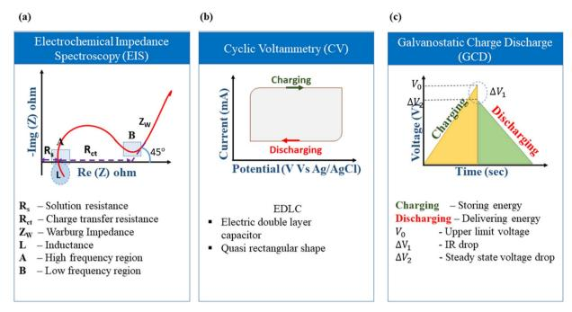
Fig. 11 Schematic of electrochemical characterization techniques: (a) EIS (b) CV and (c) GCD
