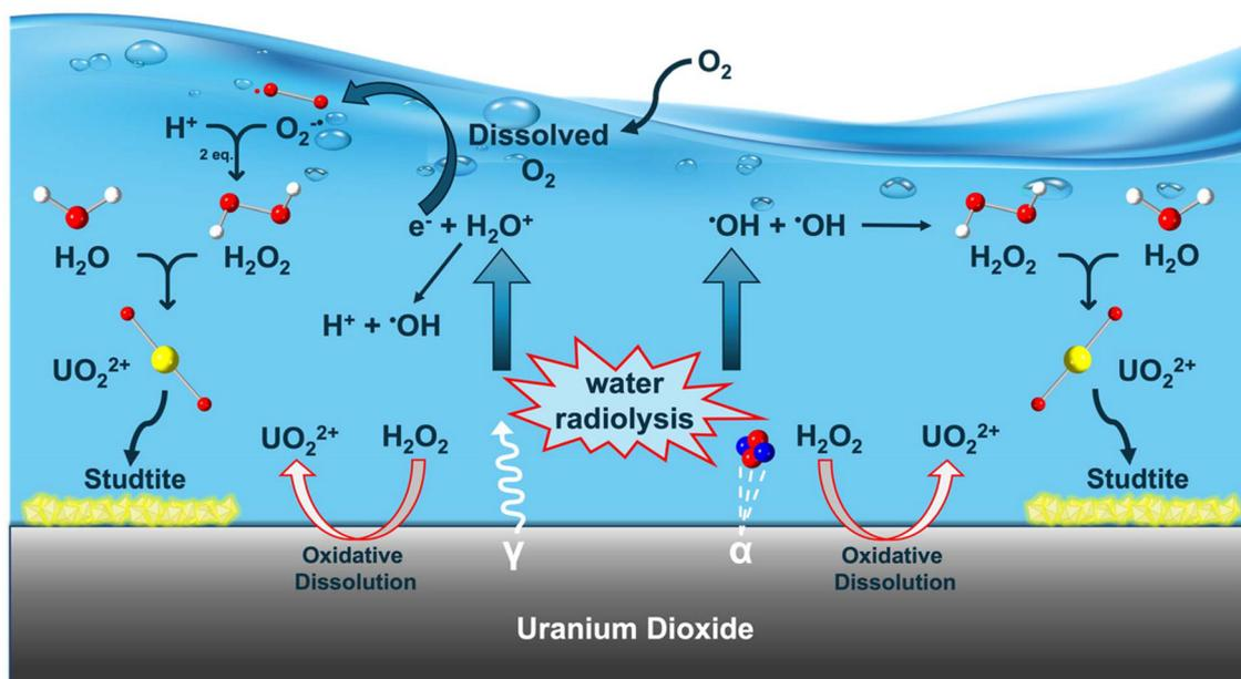
**Fig. 16** Diagram of the formation of studtite from the oxidative dissolution of UO<sub>2</sub> from water radiolysis including both  $\gamma$ - and  $\alpha$ -incident radiation pathways. Adapted from Perrot *et al.*<sup>285</sup>
