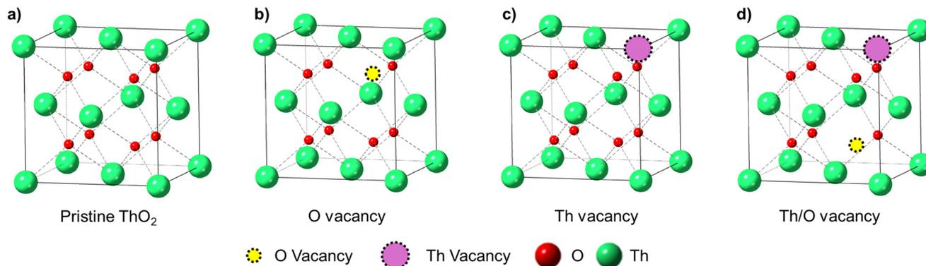
**Fig. 13** Modified figure from Park *et al.*,<sup>224</sup> shows (a) the pristine  $\text{ThO}_2$  unit cell. Radiation can result in the formation of a (b) F-center defect that can perturb the lattice to create (c) Frenkel defects. These disruptions to the lattice can create (d) dislocation loops.
