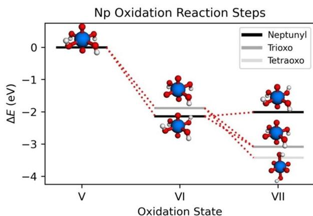
**Fig. 8** Diagram describing the formation of a stable Np(VII) species from Np(V) oxidation under basic conditions that was originally proposed by Kravchuk *et al.*<sup>74</sup> The  $\cdot\text{OH}$  was determined to be the most likely oxidant and two metastable Np(VI) complexes were identified before oxidation to the Np(VII) occurs. Np, O, and H are depicted as blue, red, and white spheres, respectively.
