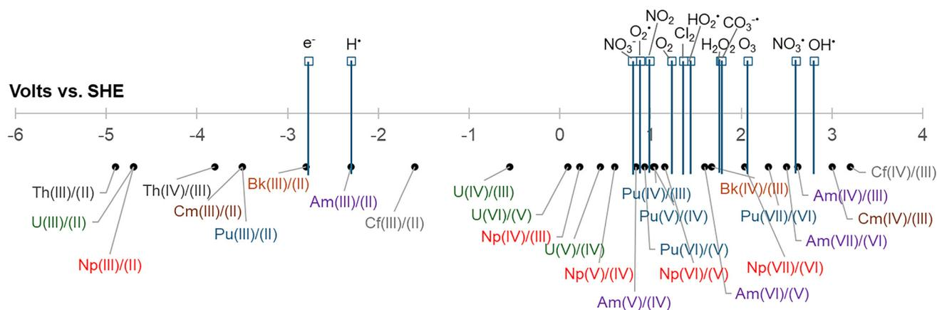
**Fig. 3** Standard reduction potentials versus the Standard Hydrogen Electrode (SHE) for free radicals produced during the radiolysis of water and aqueous solutions of common solutes compared to the common oxidation states for the actinide elements under acidic conditions.<sup>42</sup>
