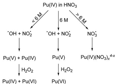
**Scheme 2** Concentration dependence of  $\alpha$ -particle irradiated  $\text{HNO}_3$  solutions leads to the formation of  $\text{Pu(IV)}$ ,  $\text{Pu(V)}$ , and/or  $\text{Pu(VI)}$ .<sup>151,152</sup>
