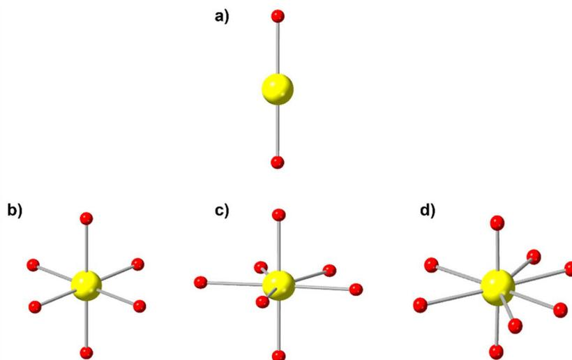
**Fig. 6** Ball-and-stick models of the hexavalent and pentavalent (a) uranyl cation ( $\text{UO}_2^{2+}/\text{UO}_2^+$ ) and potential geometries—(b) tetragonal, (c) pentagonal, and (d) hexagonal bipyramids—that are found in solution and solid-state materials. Adapted from Plášil.<sup>70</sup>
