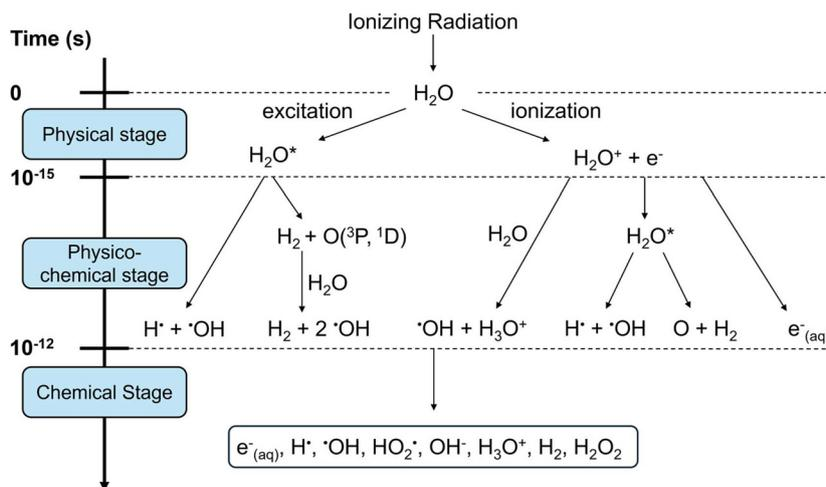
Fig. 1 Reaction scheme for the radiolysis of neat water.<sup>31</sup>
