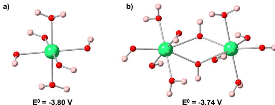
Fig. 4 Ball and stick models of (a)  $\text{Th}(\text{OH})_4(\text{H}_2\text{O})_2$  and (b)  $\text{Th}_2(\text{OH})_8(\text{H}_2\text{O})_4$  molecular hydrolysis products with their calculated reduction potentials. H, O, and Th atoms are colored pink, red, and green spheres, respectively.<sup>48</sup>
