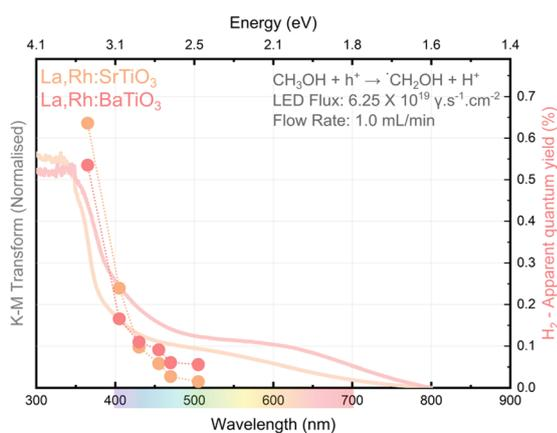
Fig. 9 Kubelka–Munk transform of UV-Vis diffuse reflectance and wavelength dependence on apparent quantum yield (AQY) of  $\text{La,Rh:SrTiO}_3$  and  $\text{La,Rh:BaTiO}_3$  from 365–505 nm. 7 mg photocatalyst, varying LED wavelength, constant photon flux ( $6.25 \times 10^{19} \gamma \text{ s}^{-1} \text{ cm}^{-2}$ ).
