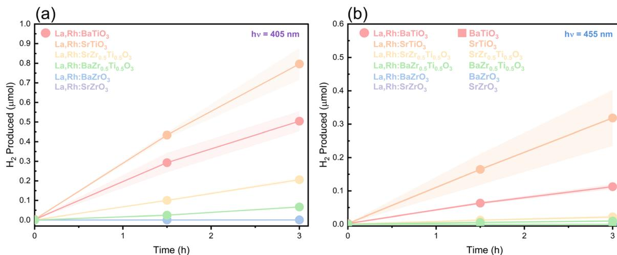
Fig. 8 Photocatalytic H<sub>2</sub> evolution of various perovskites from a 1 : 1 H<sub>2</sub>O and CH<sub>3</sub>OH mix using 405 (a) and 455 nm light (b). The shaded areas depict standard error. Conditions: 7 mg photocatalyst, 405 (228.0 mW cm<sup>-2</sup>) or 455 (88.4 mW cm<sup>-2</sup>) nm LED.
