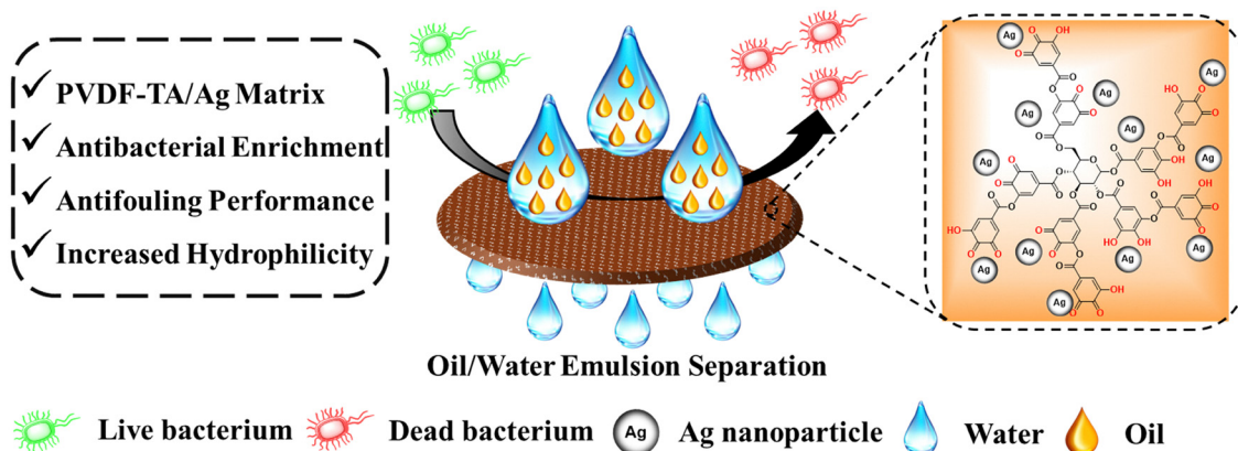
Fig. 1 Schematic representation of the newly developed tannic acid-infused silver nanoparticle-decorated PVDF membrane explicating superior antibacterial activities and enhanced oil-in-water separation.
