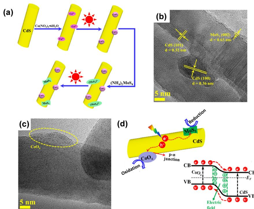
Fig. 5 (a) Schematic diagram of CdS-CoO<sub>x</sub>-MoS<sub>2</sub> nanocomposite preparation. (b) and (c) HRTEM image of CdS-CoO<sub>x</sub>-MoS<sub>2</sub> nanocomposite. (d) Proposed charge transfer mechanisms at CdS-CoO<sub>x</sub> and CdS-MoS<sub>2</sub> interfaces. Reproduced from ref. 45 with permission from [Elsevier], copyright [2022].
