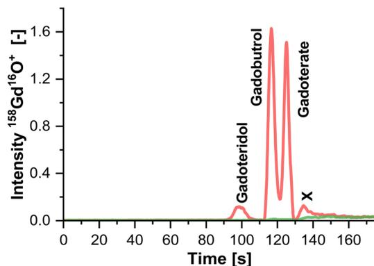
Fig. 3 IC-ICP-MS chromatogram of the sample Emr2 from the river Emscher (red) and a blank injection (green).  $^{158}\text{Gd}^{16}\text{O}^+$  intensity is normalised with the PCIS. Peaks are assigned to GBCAs and an unknown species X was detected.
