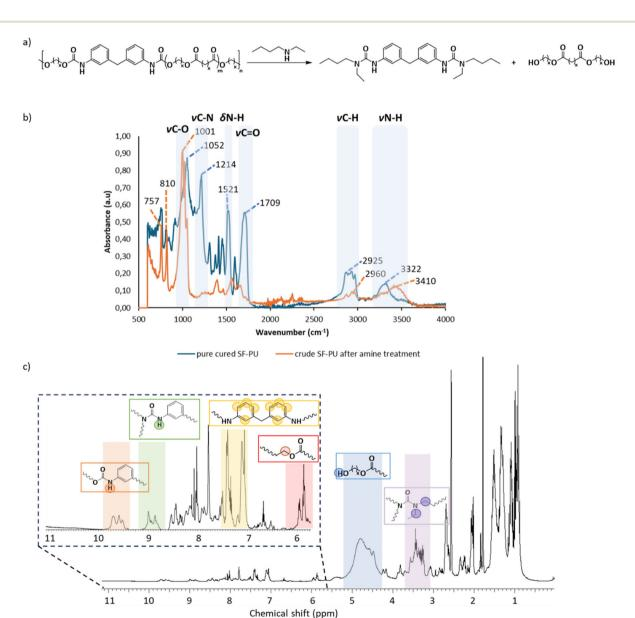
Fig. 2 (a) Chemical reaction scheme of aromatic polyester polyurethane (PU) with N-ethyl N-butyl amine (EBA); (b) FTIR spectra of the aromatic polyester polyurethane (PU) adhesive before and after EBA treatment; (c) NMR spectrum of the aromatic polyester polyurethane (PU) adhesive after EBA treatment.
