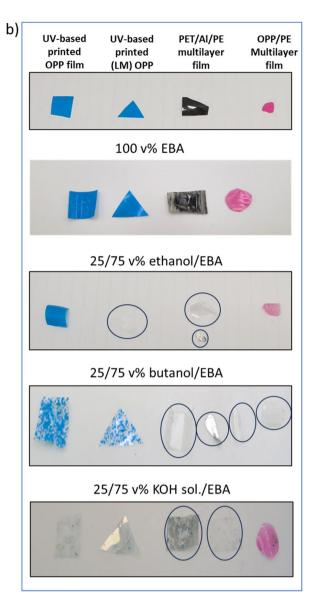
Fig. 5 Deinking and delamination of 4 different plastic films (a) in cyclohexane/N-ethyl N-butyl amine (EBA) mixture at different volume ratios; (b) in ethanol/EBA, butanol/EBA and KOH solution/EBA mixtures at 25/75 v% ratio after 4 h contact at 60 °C. Hourly visual progression of deinking and delamination of these samples in each medium is given in Fig. S5.
