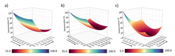
Fig. 4 Response surfaces of the delamination % as a function of (a) temperature (°C) and particle size (cm); (b) temperature (°C) and S/L ratio (q mL<sup>-1</sup>); (c) particle size (cm) and S/L ratio (g mL<sup>-1</sup>) for delamination of sample 7 through selective aminolysis of the PU adhesive layer. Delamination percentages exceeding 100% fall within the experimental error margin of the RSM model and are normalized to 100%.
