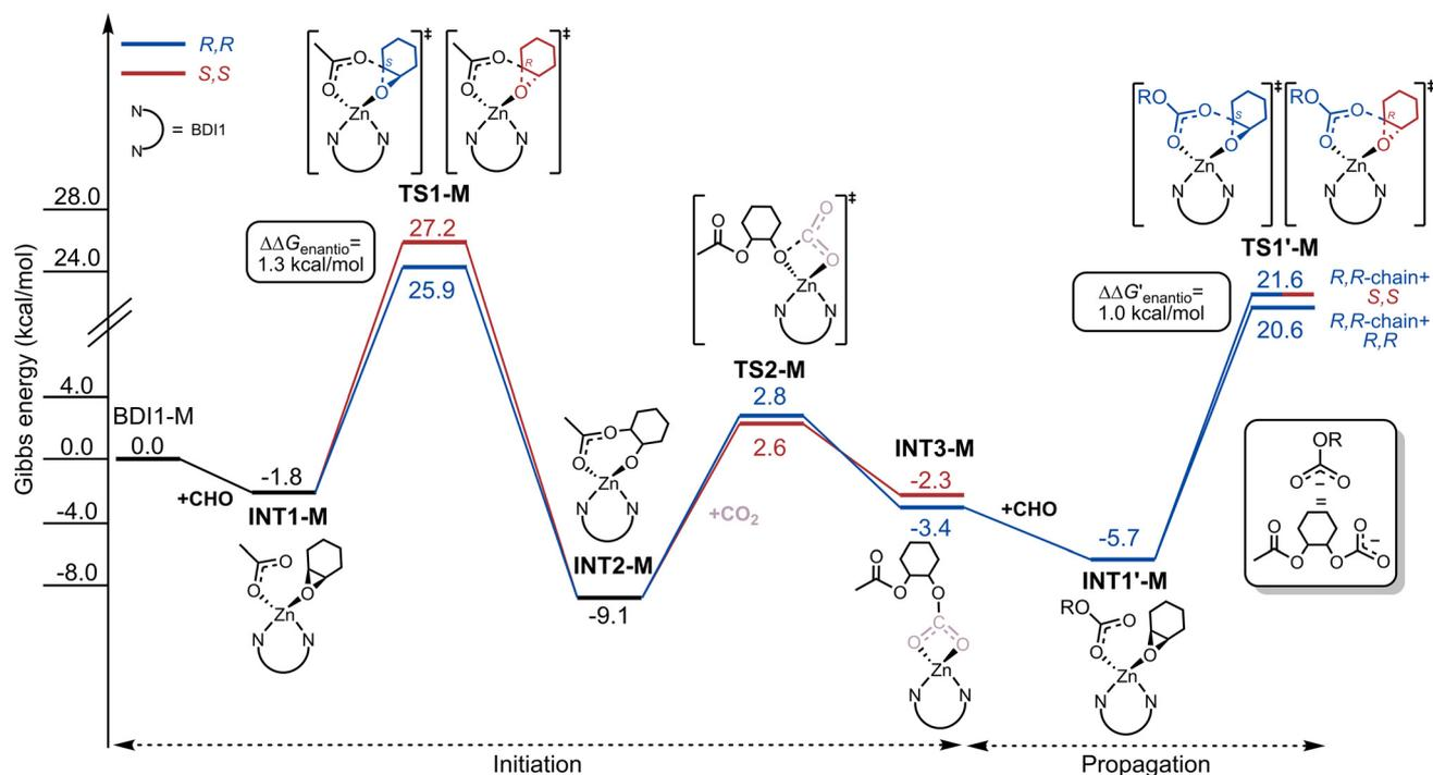
**Fig. 1** Gibbs energy profile for initiation and propagation steps in the  $\text{CHO}/\text{CO}_2$  copolymerization catalyzed by **BDI1-M**. The blue and red pathways correspond to the formation of *R,R*- and *S,S*-configured chains based on attacks on the *S* and *R* carbons of CHO, respectively. The presence of an entire growing unit ((OR) $\text{CO}_2^-$ ) is simulated in the propagation.
