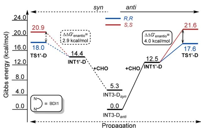
**Fig. 5** Gibbs energy profile for the CHO ring-opening on an *R,R*-configured growing unit, by BDI1-D<sub>syn</sub> (left) and BDI1-D<sub>anti</sub> (right). Energies (kcal mol<sup>-1</sup>) are calculated with respect to the more stable INT3-D<sub>anti</sub> species. The paths leading to a second *R,R*-chain and *S,S*-chain formation are reported, respectively, in blue and red.
