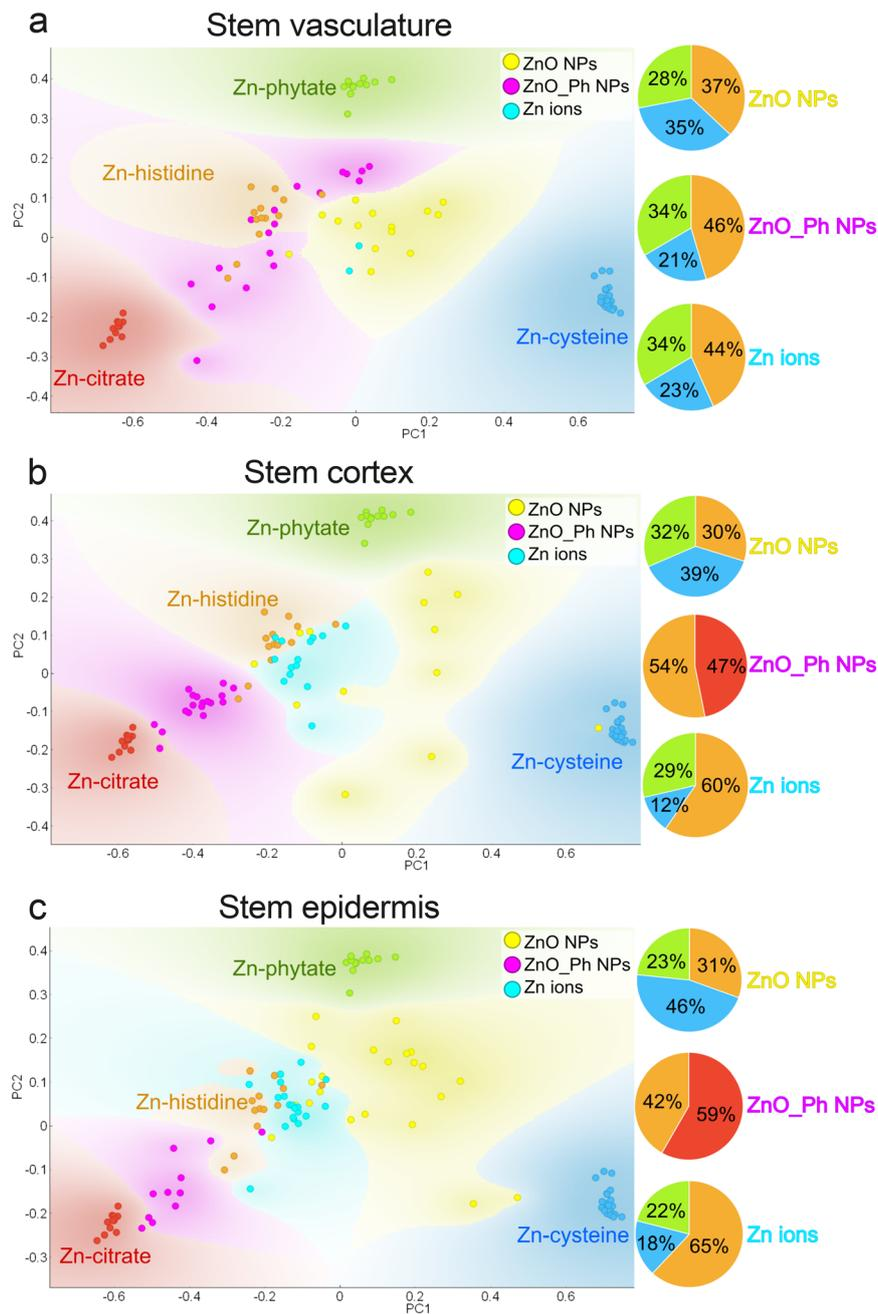
**Fig. 5** PCA of XANES collected on selected POIs in the stem (a) vasculature, (b) cortex and (c) epidermis of pepper plants exposed to ZnO\_Ph NPs, ZnO NPs or Zn ions 1 week after exposure. The following references were used for comparison: Zn-cysteine in blue (Zn-thiol), Zn-citrate in red (Zn-carboxyl), Zn-phytate in green (Zn-phosphate) and Zn-histidine in orange (Zn-carboxyl). Eigenvalue for (a) PC1: 0.77 and PC2: 0.16, (b) PC1: 0.79 and PC2: 0.15 and (c) PC1: 0.77 and PC2: 0.16.
