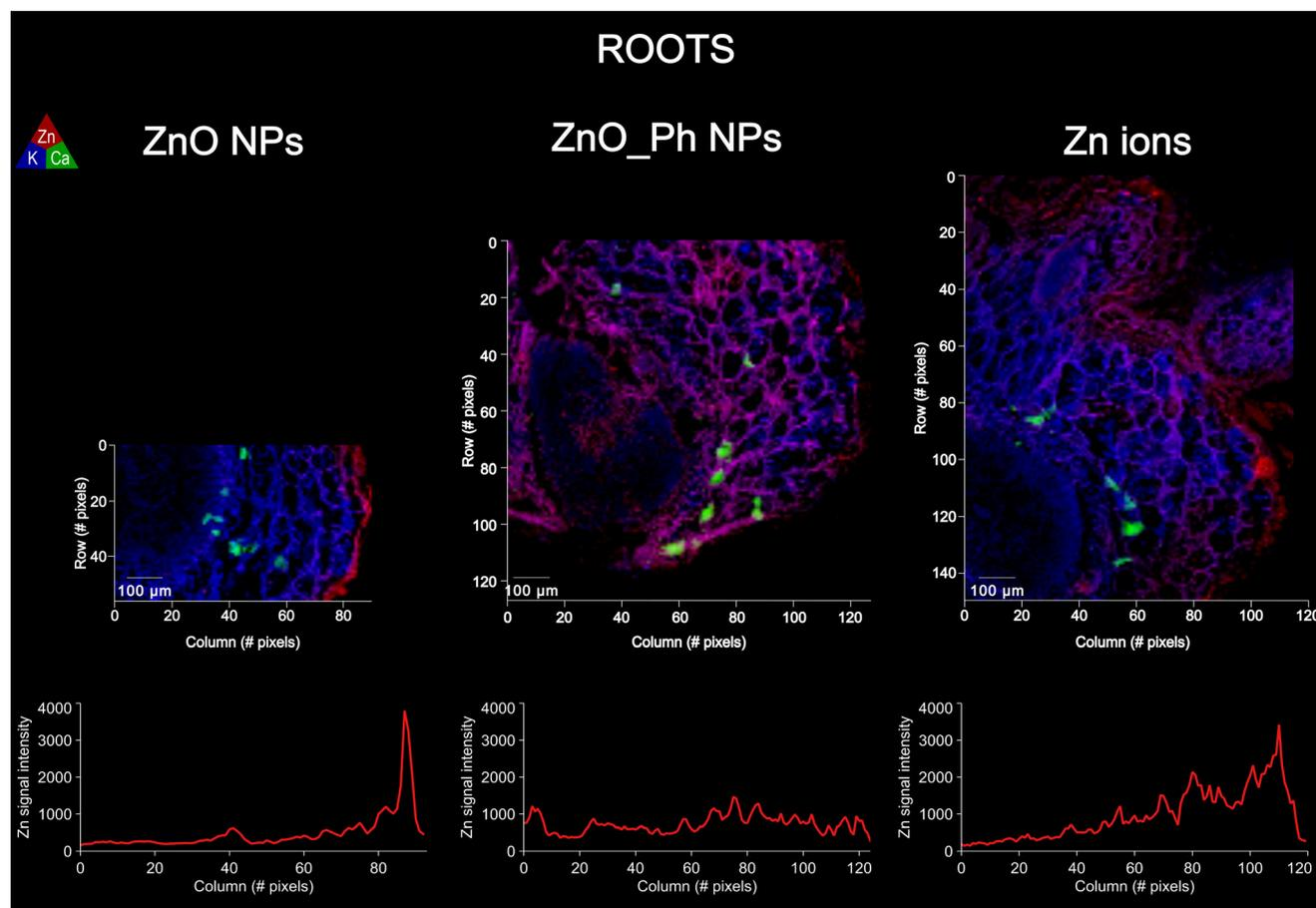
**Fig. 2** Elemental  $\mu$ -XRF maps on roots of pepper plants exposed to ZnO NPs, ZnO\_Ph NPs and Zn ions: one week after exposure. The  $\text{K}\alpha$  fluorescence of Zn is represented in red, K in blue and Ca in green. Below each  $\mu$ -XRF map is the average fluorescence intensity measured for Zn along a selected root cross-section. The averaging of Zn  $\text{K}\alpha$  fluorescence intensity was performed by averaging 3 profiles per  $\mu$ -XRF map (Fig. S3<sup>†</sup>).
