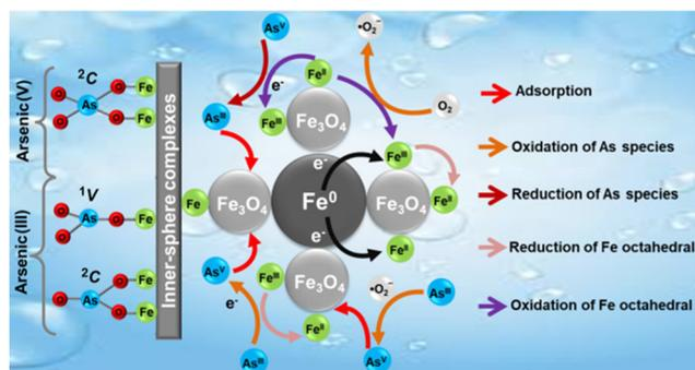
Fig. 11 Mechanism of arsenic removal *via* bimetal oxide materials.<sup>126</sup>
