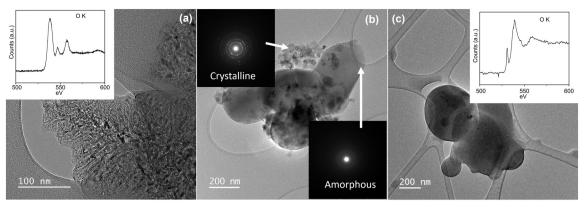
Fig. 3 Representative images of MgO carbonation. (a) MgO was prepared by calcinating mined MgCO<sub>3</sub> and freshly dispersed on a TEM grid (day-0), inset: O K EELS spectra. (b) MgO aggregate dispersed on a TEM grid undergoing carbonation, inset: selected area electron diffraction (SAED) pattern from the carbonated and uncarbonated region. (c) Fully carbonated MgO aggregate (MgCO<sub>3</sub>) dispersed on a TEM grid, inset: O K EELS spectra of fully carbonated aggregates.
