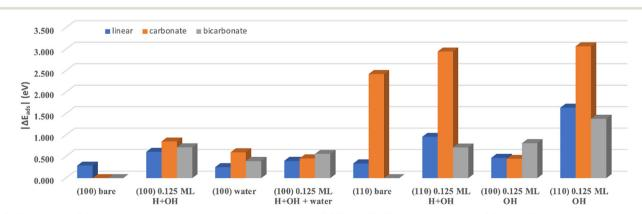
Fig. 9 The lowest CO2 adsorption energy on bare and functionalized (100) and (010) surfaces with the CO2 in different configurations: linear, carbonate and bicarbonate.
