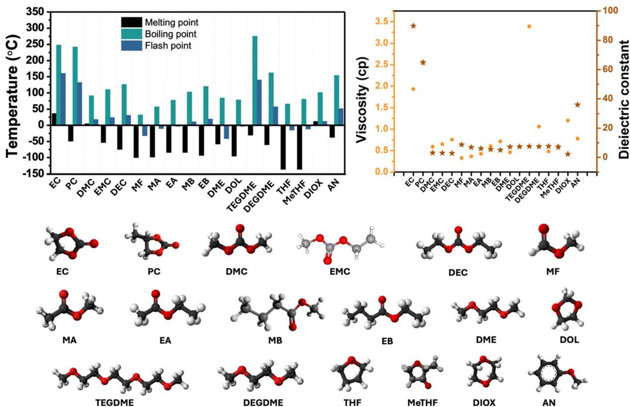
Fig. 6 Comparison of physical properties of selected solvents.
