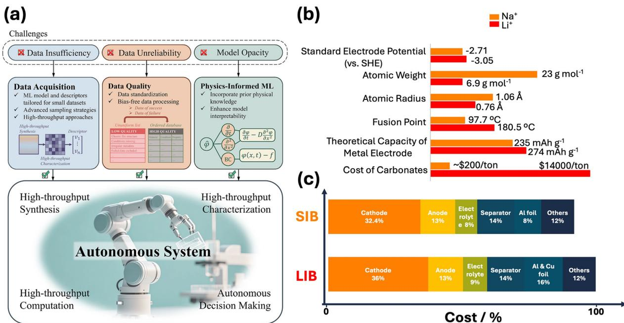
**Fig. 15** (a) Overcoming key challenges and realizing opportunities through AI in rechargeable battery materials design.<sup>250</sup> (b) Comparison of sodium and lithium properties, and (c) the manufacturing costs for LIB and SIB cell components.
