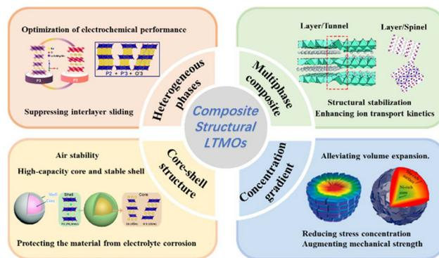
Fig. 1 Schematic diagram of composite structural LTMO design in SIBs.
