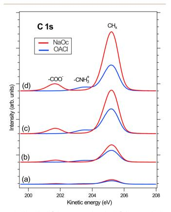
Fig. 5 Normalized C 1s spectra to the related O 1s spectra in the presence of (a) pure water, (b) NaCl 50 mM, (c) NaCl 426 mM, and (d) ASW 520 mM. The intensity of the spectra was normalized to that of the  $\rm H_2O(I)$  peak in the respective O 1s spectra.
