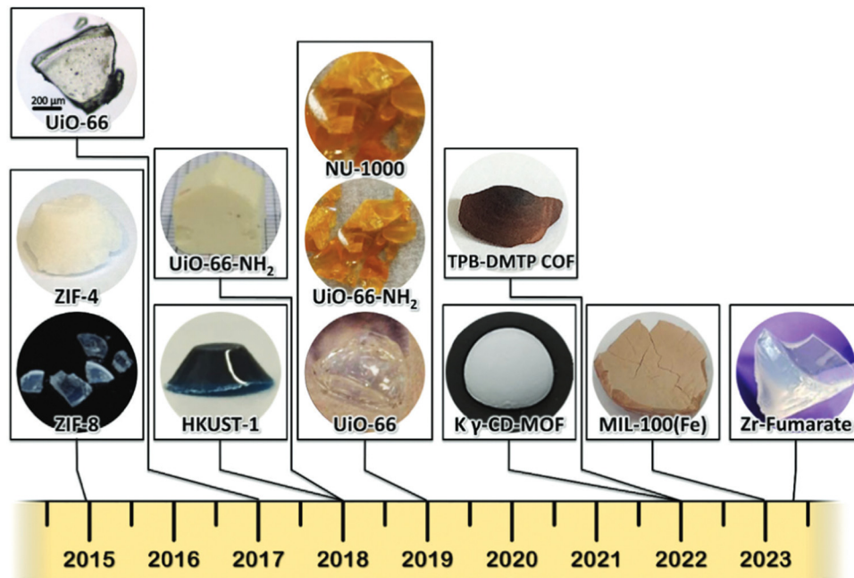
Fig. 9 Chronological overview of sol-gel monoliths, accompanied by optical images, illustrating the self-shaping evolution of key monolithic MOFs and COFs. Reproduced with permission from ref. 127 Copyright 2023 Wiley.
