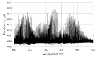
Fig. 3 Overview spectrum of  $C_2H_3DO$  as recorded for this study. (T = 295 K,  $P \approx 1.8$  mbar, resolution = 0.0015 cm<sup>-1</sup>, l = 18 cm). Decadic absorbance  $\lg(I_0/I)$  is shown (partial pressure, see text).
