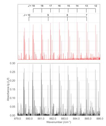
Fig. 8 Comparison of measured (black) and calculated (red) P branch transitions in the  $\nu_{12}$  fundamental of  $c\text{-}C_2H_3DO$ . The assignments are shown in the figure. Transitions associated with J = 12-19 in the  $K_a = 0$ series (upper comb) and with J = 7-10 in the  $K_c = 0$  series (lower comb) are shown. Decadic absorbance is shown  $lg(I_0/I)$ .
