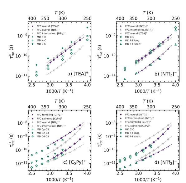
Fig. 4 Temperature-dependent rotational correlation times τ<sub>rot</sub> of <sup>1</sup>H carrying cations (a) and (c) and <sup>19</sup>F carrying anions (b) and (d) for the ionic liquids  $[TEA][NTf_2]$  (a) and (b) and  $[C_5Py][NTf_2]$  (c) and (d). Values from FFC NMR relaxometry are shown as purple filled symbols. Values from MD simulations are shown as green open symbols. Subfigures with cation data include anion data as gray symbols and vice versa.
