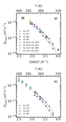
Fig. 5 Temperature-dependent self-diffusion coefficients  $D_{\rm H}$  for cations and  $D_E$  for anions in the ionic liquids [TEA][NTf<sub>2</sub>] (a) and [C<sub>5</sub>Py][NTf<sub>2</sub>] (b). Values from FFC NMR relaxometry are shown as purple filled symbols. Values from MD simulations are shown as green open symbols
