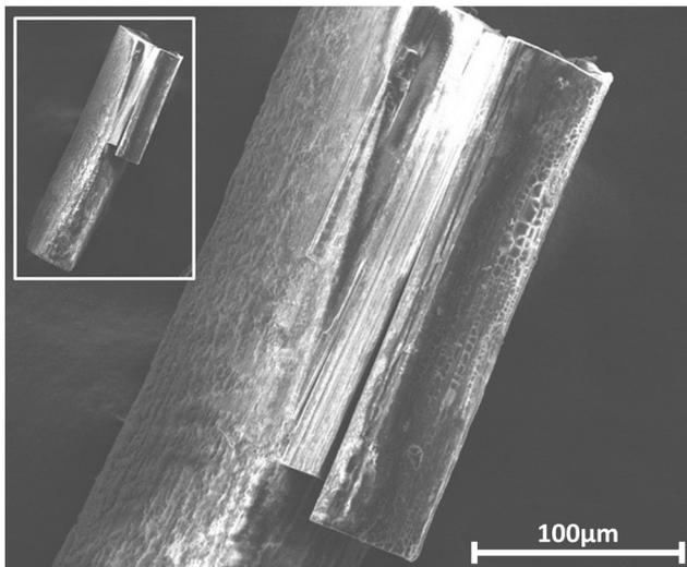
**Fig. 3** Scanning Electron Microscope (SEM) image obtained using a high-resolution Hitachi S4800 equipment (scale at the bottom right), showing the characteristic needle-like morphology of a small single crystal of synthetic nesquehonite, provided by the Yale Peabody Museum (specimen YPM MIN 031567). The sample was originally synthesized by Genth and Penfield<sup>21</sup> over a century ago. The inset shows the entire analyzed crystal.
