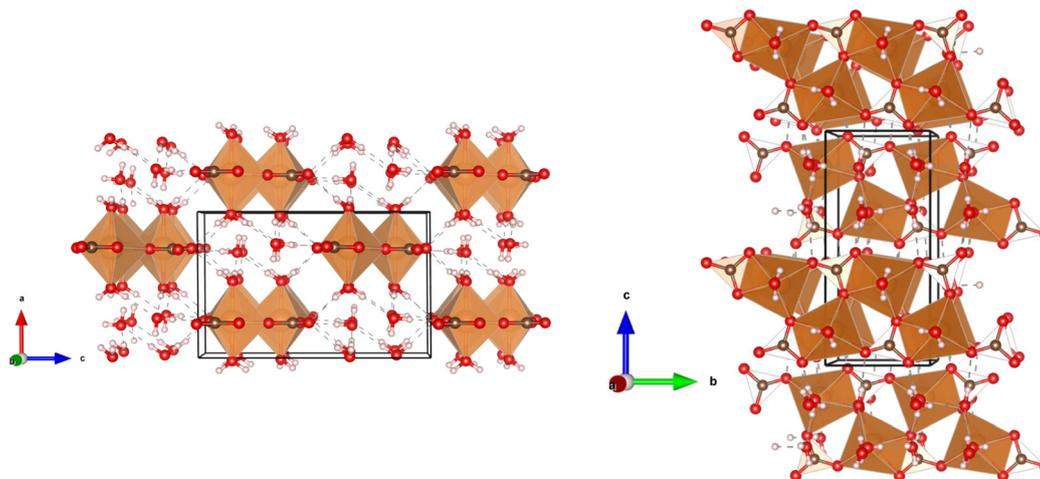
**Fig. 2** Projection of  $\text{MgCO}_3 \cdot 3\text{H}_2\text{O}$  nesquehonite along the  $b$ -axis (left) and  $a$ -axis (right) at room conditions. Magnesium (Mg), oxygen (O), carbon (C), and hydrogen (H) atoms are represented in orange, red, brown, and white, respectively.
