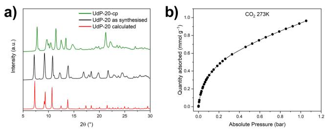
Fig. 3 PXRD pattern comparison between UdP-20 calculated (red), UdP-20 as synthesised and UdP-20 after the activation process (UdP-20-cp, green) (a). CO<sub>2</sub> isotherm at 273 K registered on UdP-20-cp (b).
