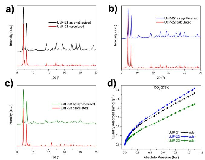
Fig. 6 Experimental and calculated PXRD patterns (a)-(c) and CO<sub>2</sub> isotherms at 273 K (d) of UdP-21, UdP-22 and UdP-23
