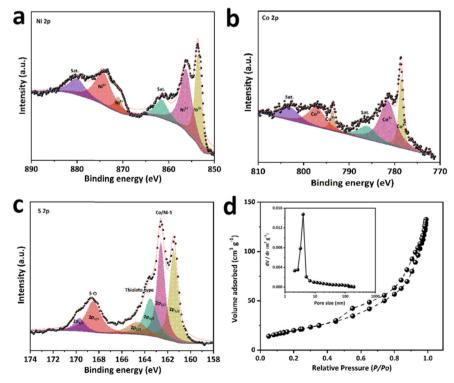
Fig. 2 (a) Ni 2p, (b) Co 2p and (c) S 2p XPS spectra of the CoNi<sub>2</sub>S<sub>4</sub>/NiS<sub>2</sub> hollow architectures; (d) N<sub>2</sub> adsorption/desorption isotherms and the corresponding pore size distributions (inset) of the CoNi<sub>2</sub>S<sub>4</sub>/NiS<sub>2</sub> hollow architectures.
