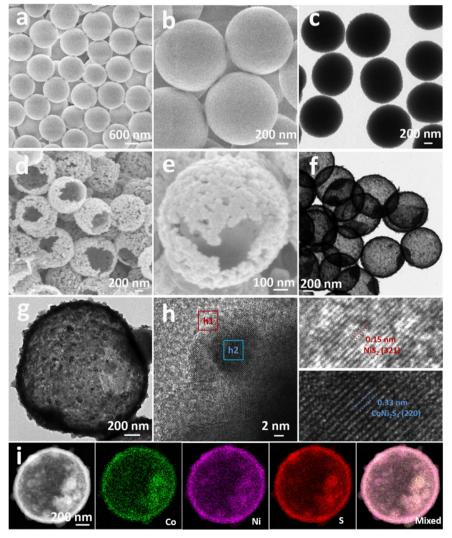
Fig. 1 (a and b) FESEM and (c) TEM images of Ni–Co glycerate, (d and e) FESEM and (f and g) TEM images of  $CoNi_2S_4/NiS_2$  hollow architectures, (h and i) HRTEM and TEM elemental mapping images of  $CoNi_2S_4/NiS_2$  hollow architectures.
