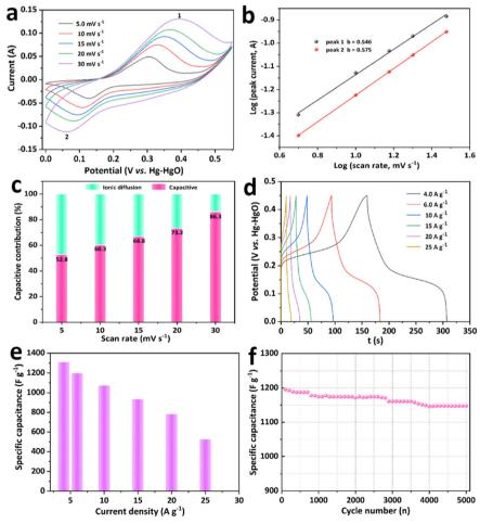
Fig. 3 Electrochemical behavior of the  $CoNi_2S_4/NiS_2$  hollow architectures as supercapacitors: (a) CV curves at scanning rates of 5.0 to 30 mV s<sup>-1</sup>; (b) the linear relationships between log (peak currents) and log (scanning rates); (c) capacitive contribution ratios at various scanning rates; (d) GCD; and specific capacitance profiles (e) at various current densities; (f) continuous cycling performance at 6.0 A g<sup>-1</sup> after 5000 cycles.
