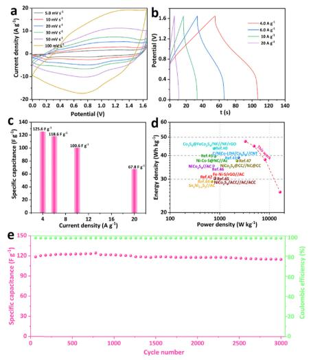
Fig. 4 Electrochemical performance of the two-electrode system: (a) CV profiles at scanning rates of 5.0 to 100 mV s<sup>-1</sup>; (b) GCD profiles in current densities of 4.0 to 20 A g<sup>-1</sup>; (c) specific capacitance at various current densities; (d) Ragone plots; and (e) cycling stability for 3000 cycles at 6.0 A g<sup>-1</sup>.
