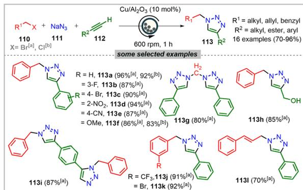
**Scheme 20** Cu/Al<sub>2</sub>O<sub>3</sub>-catalysed, solvent-free, one-pot synthesis of 1,2,3-triazoles starting from alkyl halides, sodium azide, and alkynes under ball-milling.
