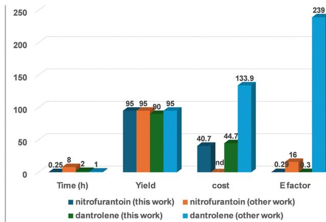
**Fig. 9** Comparison of time, yield, cost, and *E*-factor between previous work and the present work for the synthesis of nitrofurantoin and dantrolene.
