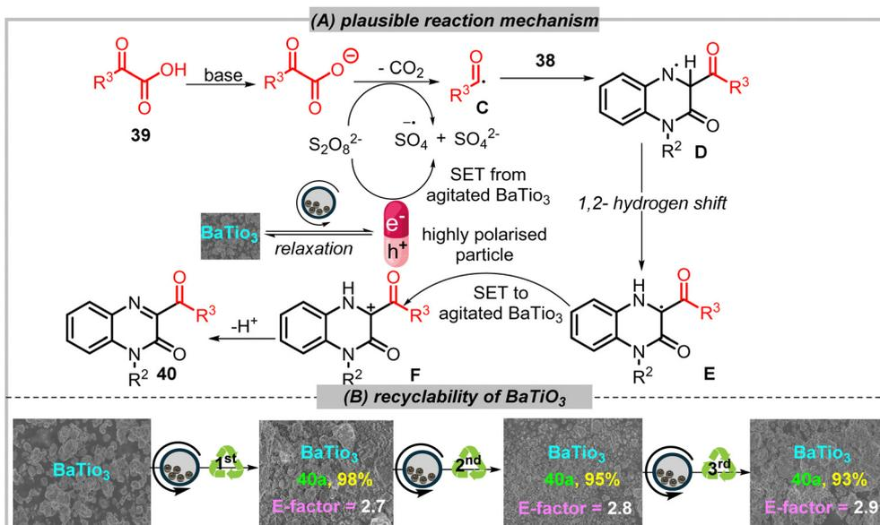
Scheme 8 (A) Proposed mechanism for decarboxylative acylation of quinoxaline. (B) Recycling efficiency of the piezocatalyst, BaTiO<sub>3</sub>.
