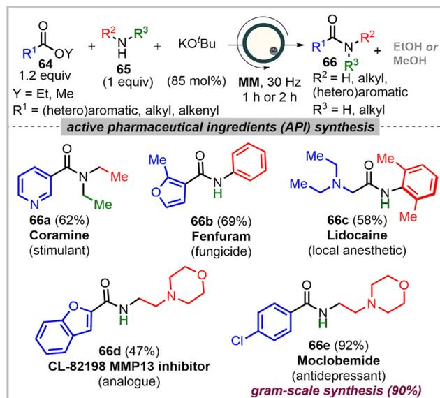
Scheme 11 Amidation of esters via solvent-free ball-milling.
