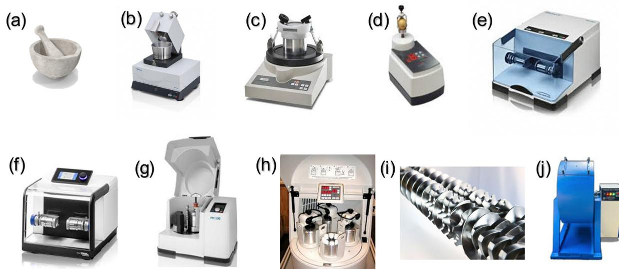
**Fig. 1** Typical grinding and milling equipment: (a) mortar and pestle, (b) Retsch automated mortar, (c) Fritsch vibrational mill, (d) Fritsch vertical shaker mill, (e) Retsch vibrational ball mill, (f) Retsch vibrational ball mill with controlled temperature (cryomill), (g) Retsch planetary ball mill, (h) multiple-sample mill (automaxion), (i) twin-screw used for continuous mechanochemical extrusion, and (j) tumbler ball-mill.
