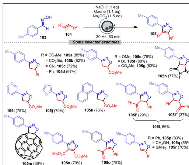
**Scheme 19** Solvent-free synthesis of isoxazoles under ball milling.
