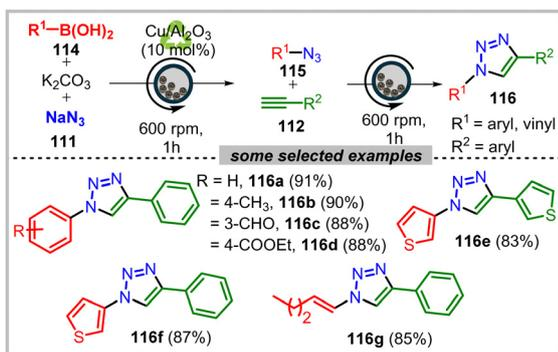
**Scheme 21** Cu/Al<sub>2</sub>O<sub>3</sub>-catalysed, solvent-free, one-pot synthesis of 1,2,3-triazoles starting from boronic acids, sodium azide, and alkynes under ball-milling.
