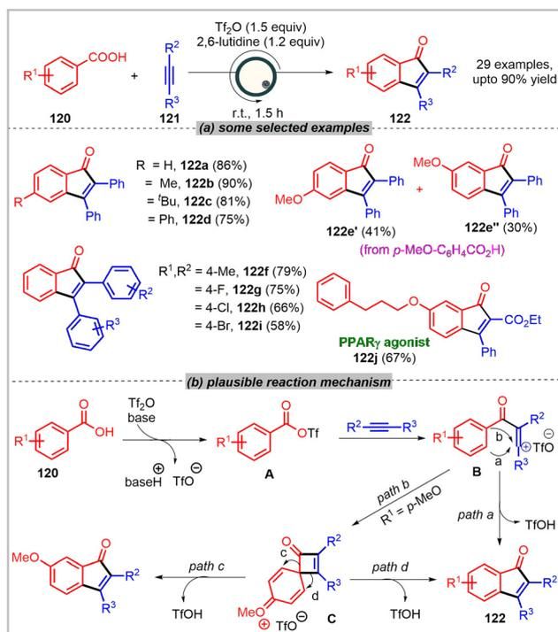
**Scheme 22** (a) Some selected examples for the solvent-free mechanochemical synthesis of pharmaceutically active indenones under ball milling, and (b) the plausible reaction mechanism.
