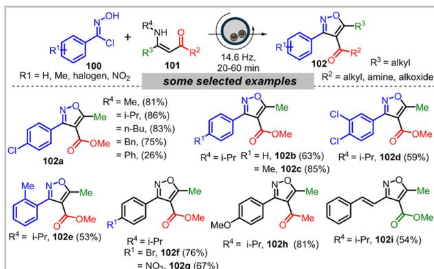
**Scheme 17** Solvent-free synthesis of isoxazoles from *N*-hydroxybenzimidoyl chlorides and enamines under ball milling.
