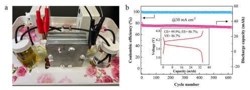
Fig. 10 (a) A photograph of the neutral Zn/Fe RFB stack. (b) Cycling performance of the cell stack; the inset shows the 10th charging/discharging curve [reproduced with permission from ref. 64].
