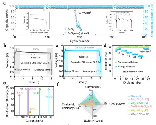
Fig. 9 (a) Long-term cycling tests of the Zn-Fe RFB at 20 mA cm<sup>-2</sup>. (b) and (c) Long standby tests of the Zn-Fe RFB using pure ZnCl<sub>2</sub> and ZnCl<sub>2</sub>-NAM. (d) Rate performance of the Zn-Fe RFB adopting a mixed ZnCl<sub>2</sub> and NAM anolyte at 10-50 mA cm<sup>-2</sup>. (e) and (f) Comparison of the proposed Fe-Zn flow cell with other reported Zn-based RFBs [reproduced with permission from ref. 70].
