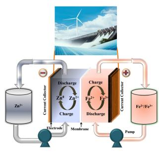
Fig. 3 Working principle of the Zn-Fe redox flow battery.
