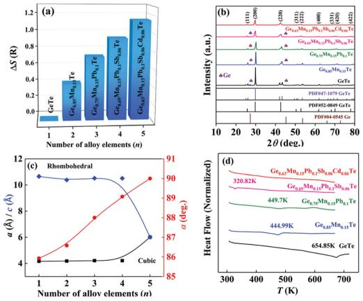
Fig. 21 (a) Configurational entropy ΔS, (b) powder XRD patterns, (c) lattice parameter a/c and interaxial angle,  $\alpha$ , at 300 K, of GeTe-based alloys, and (d) DSC curves showing the lowering of the phase transition temperature of medium entropy GeTe-based alloys. Reproduced and adapted from ref. 154  $\odot$  2021 The Authors. Advanced Science published by Wiley-VCH GmbH under the terms of the Creative Commons CC BY license.
