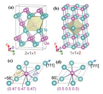
Fig. 2 Characteristics of the GeTe alloy as a thermoelectric material. Crystal structures of (a) rhombohedral GeTe and (b) cubic GeTe along with the respective primitive cells of (c) rhombohedral GeTe and (d) cubic-GeTe. Reproduced with permission from © 2019 Wiley-VCH Verlag GmbH & Co. KGaA, Weinheim.51
