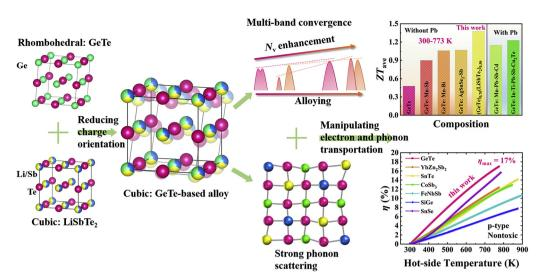
Fig. 12 Schematic demonstration of the origin of crystal structure and the factors responsible for enhanced thermoelectric performance of the GeTederivatives. Reproduced and adapted from ref. 142, under the Creative Commons CC-BY-NC-ND license.
