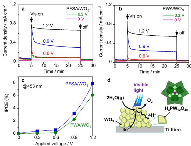
**Fig. 5** Effect of applied voltage (*V* vs. Pt–CB cathode) on the photocurrent response of (a) PFSA/WO<sub>3</sub> and (b) PWA/WO<sub>3</sub> in the vapour-fed PEM-PEC system under visible light (453 nm, 22 mW cm<sup>-2</sup>). (c) Steady-state IPCE at 453 nm after 20 min of photoirradiation. (d) Schematic illustration of PEC triple-phase boundary over the PWA/WO<sub>3</sub> photoanode. The loading of PWA and PFSA were 5 and 12 wt% relative to WO<sub>3</sub>.
