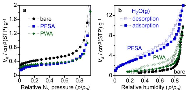
**Fig. 6** (a) Nitrogen adsorption isotherms at -196 °C and (b) water vapour adsorption-desorption isotherms at 25 °C for bare WO<sub>3</sub>, PWA/WO<sub>3</sub>, and PFSA/WO<sub>3</sub> layers on Ti felt. The loading of PWA and PFSA were 5 and 12 wt% relative to WO<sub>3</sub>.
