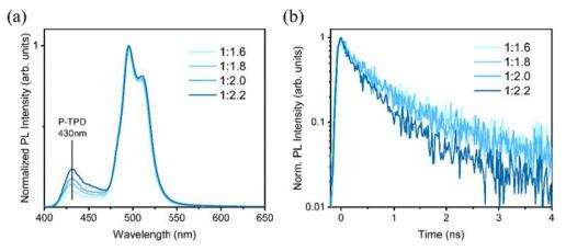
Fig. 6 (a) Normalized PL spectra and (b) time-resolved photoluminescence measurement (495 nm) of the composite film prepared by constant NPLs concentration (15 mg mL<sup>-1</sup>) and NPLs to P-TPD ratio of 1:1.6, 1:1.8, 1:2.0, and 1:2.2.
