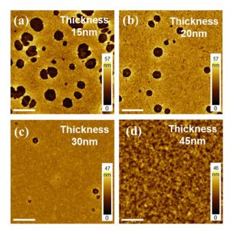
Fig. 5 Under a fixed concentration of NPLs (15 mg mL<sup>-1</sup>) and a ratio of NPL to P-TPD (1:2), AFM surface morphologies of the blade-coated films with different thicknesses of (a) 15 nm, (b) 20 nm, (c) 30 nm, and (d) 45 nm. All white scale bars represent 2 µm.
