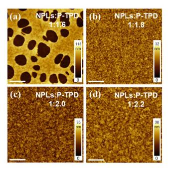
Fig. 4 AFM images showing surface morphologies of the blade-coated films using a solution with constant NPL concentration (15 mg  $mL^{-1}$ ) and NPLs to P-TPD ratio of (a) 1:1.6, (b) 1:1.8, (c) 1:2.0 and (d) 1:2.2 with a fixed thickness of 45 nm. All white scale bars represent 2  $\mu$ m.
