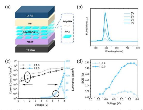
Fig. 7 (a) Device structure, (b) EL spectra of the optimized device with the active layer thickness 45 nm and prepared from a 15 mg mL<sup>-1</sup> NPL suspension with a polymer mixing ratio of 1:2. (c) Current density-luminance-voltage curves and (d) EQE-V curves of sky-blue LED with different ratios of NPLs to P-TPD.
