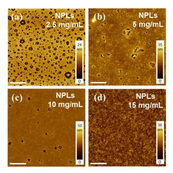
Fig. 3 AFM surface morphologies of the blade-coated composite films under fixed NPLs to P-TPD ratio (1:2), with NPL concentration of (a)  $2.5 \text{ mg mL}^{-1}$ , (b)  $5 \text{ mg mL}^{-1}$ , (c)  $10 \text{ mg mL}^{-1}$  and (d)  $15 \text{ mg mL}^{-1}$ . All white scale bars represent 2 µm.
