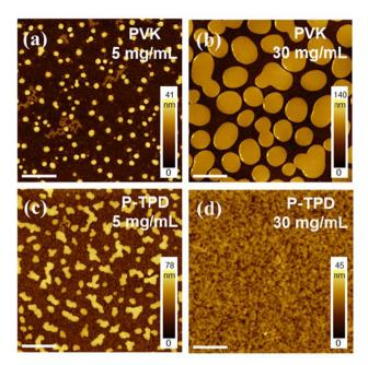
Fig. 2 AFM surface topography of the blade-coated films with different ratios of polymers at 10 mg mL $^{-1}$  NPL concentration. (a) PVK at 5 mg mL $^{-1}$ ; (b) PVK at 30 mg  $mL^{-1}$ ; (c) P-TPD at 5 mg  $mL^{-1}$  and (d) P-TPD at 30 mg mL $^{-1}$ . All the white scale bars represent 2  $\mu$ m.
