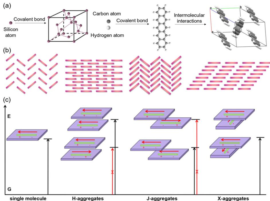
**Fig. 1** (a) Schematic illustration of the formation of a single crystal unit cell of representative inorganic semiconductors (silicon) and organic semiconductors (pentacene). (b) The four classical packing motifs for organic semiconductors. (c) The energy splitting diagrams of organic aggregates. Reproduced with permission.<sup>35</sup> Copyright 2021, John Wiley and Sons.
