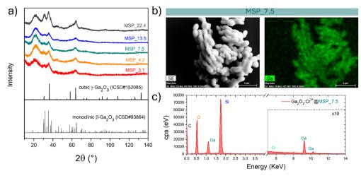
Fig. 2 (a) XRPD patterns of the samples with increasing pore size of the mesopores of the MSPs where the Ga<sub>2</sub>O<sub>3</sub> NCs were grown. (b) Representative secondary electron-SEM image and corresponding EDX elemental map of Ga and (c) EDX spectrum of the Ga<sub>2</sub>O<sub>3</sub>:Cr<sup>3+</sup>@MSP\_7.5 sample.
