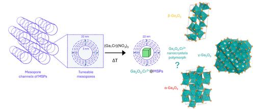
Scheme 1 Sketch of the synthetic procedure for the synthesis of  $Ga_2O_3$ :  $Cr^{3+}$  nanocrystals with tunable size inside the mesopores of MSPs by means of a wet impregnation strategy followed by thermal treatment and the most common Ga<sub>2</sub>O<sub>3</sub> polymorphs that could be stabilized.
