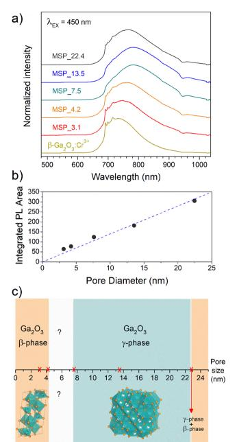
Fig. 3 (a) PL spectra of Cr<sup>3+</sup> in Ga<sub>2</sub>O<sub>3</sub> NCs grown in mesopores of different size, (b) integrated PL area as a function of the pore size and (c) diagram of the stabilized Ga<sub>2</sub>O<sub>3</sub> polymorph versus pore size.
