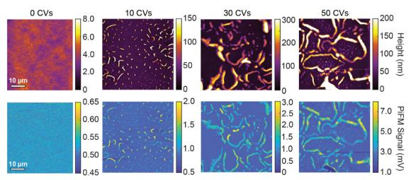
Fig. 4 AFM topography and PiFM images of a RRa P3HT thin film upon increasing numbers of CVs performed in aqueous 100 mM KTFSI after a 40 s -0.5 V (vs. Ag/AgCI) dedoping step.  $50 \times 50$   $\mu$ m AFM topography and PiFM images are collected of an undoped RRa P3HT thin film, as well as RRa P3HT thin films that underwent 0, 10, 30, and 50 CVs.
