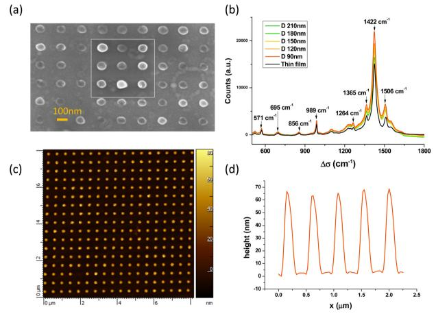
Fig. 1 (a) SEM of PEDOT/DS NP disks with an average diameter of 90 nm. (b) Raman spectra of PEDOT/DS NPs and thin-film PEDOT/DS obtained with laser irradiation of 633 nm and an acquisition time of  $3 \times 10$  s. The baseline was corrected using a polynomial fit. (c) AFM image of PEDOT/DS NP disks with an average diameter of 150 nm. (d) Height profile of PEDOT NPs.
