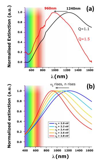
Fig. 3 (a) Normalized extinction spectra of PEDOT NPs (diameter 90 nm, height 65 nm) before (black curve) and after (red curve) acid treatment. (b) Simulation of the effect of plasma frequency, i.e. the density of chargecarriers, on the LSPR wavelength calculated using the Drude model and using  $\omega_p$  values from 2 eV to 2.8 eV.
