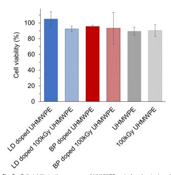
Fig. 8 Cell viability in the presence of UHMWPE and of analgesic doped UHMWPEs. The cell line MG-63 (ATCC) was exposed to the analgesic doped UHMWPEs (3  $\times$  5  $\times$  8 mm<sup>3</sup> samples, n = 3 for each group) for 24 h. Cell viability was measured with the XTT assay.
