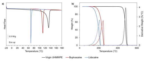
Fig. 3 Thermal and thermogravimetric behavior of UHMWPE and selected analgesic drugs. (a) DSC first heating scan and (b) TGA heating ramp  $(10 \, ^{\circ}\text{C min}^{-1})$  for virgin UHMWPE (black line), bupivacaine (red line) and lidocaine (blue line). Dashed lines in (b) refer to the derivative weight curves.
