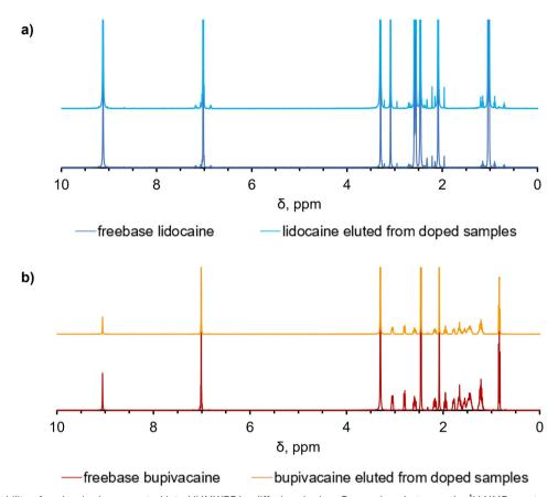
Fig. 5 Chemical stability of analgesics incorporated into UHMWPE by diffusion doping. Comparison between the <sup>1</sup>H NMR spectra of the freebase stock solution and the drug eluted from the doped UHMWPE samples for (a) lidocaine and (b) bupivacaine.
