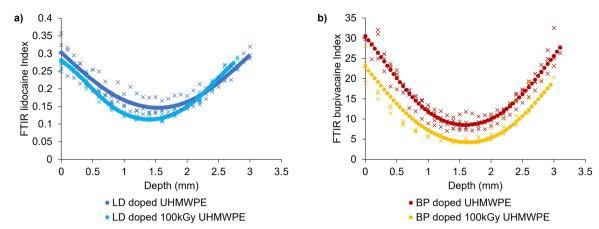
Fig. 4 Spatial distribution of lidocaine and bupivacaine in UHMWPE. Diffusion profiles along the thickness of  $3 \times 5 \times 20$  mm<sup>3</sup> prismatic strips for (a) lidocaine-doped materials and (b) bupivacaine-doped materials. Full circles represent spline interpolations of FTIR scans from multiple sections (n = 3).
