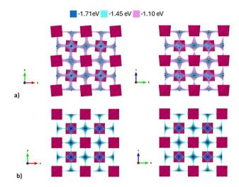
Fig. 4 BVSE isosurfaces generated from the crystal structure of the tetragonal (a) and cubic (b) phases of Na<sub>3</sub>SbS<sub>4</sub> and Na<sub>2 9</sub>Sb<sub>0 9</sub>W<sub>0.1</sub>S<sub>4</sub> respectively. The isosurfaces of constant Na<sup>+</sup> bond-valence site energy 0.26 eV and 0.61 eV above the site energy of the lowest energy Na<sup>+</sup> site are shown, with blue spheres marking the local BVSE minima representing possible Na<sup>+</sup> sites.
