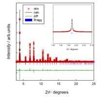
Fig. 2 Room temperature Rietveld refined synchrotron XRPD patterns of (a)  $Na_3SbS_4$  and (b)  $Na_2.9Sb_{0.9}W_{0.1}S_4$ , showing in the inset the splitting of a selected peak (2 2 0) for the tetragonal polymorph (a).
