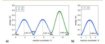
Fig. 3 Migration energy profiles as derived from BVSE analysis of the synchrotron diffraction data for tetragonal  $Na_3Sb_1S_4$  (a) and cubic  $Na_2.9Sb_0.9W_{0.1}S_4$  (b).
