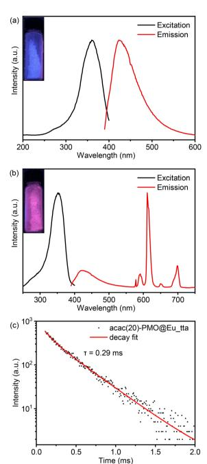
Fig. 2 (a) Combined RT excitation-emission spectrum of the acac(20)-PMO (excited at 360 nm observed at 420 nm); (b) combined RT excitation-emission spectrum of the acac(20)-PMO@Eu\_tta, ex = 352 nm, em = 611 nm; (c) luminescence decay profile of as prepared acac(20)-PMO@Eu\_tta, ex = 352 nm, em = 611 nm. Measurements refer to the sample in solid form
