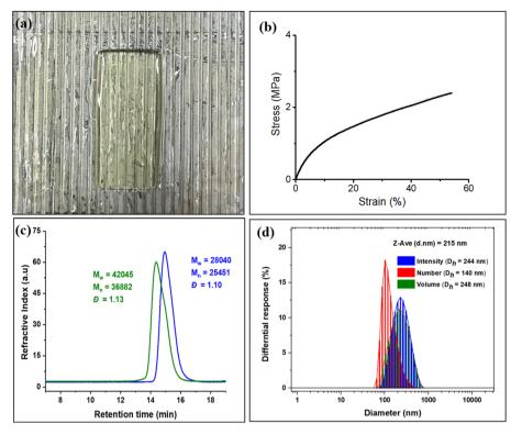
Fig. 8 (a) Resin formed from the polymer after removing the air bubbles. (b) Stress-Strain curve of the printed bars. (c) GPC traces for triblock copolymer synthesized by using EuO, EGE with CO<sub>2</sub> (green color) and GPC of copolymer of EuO with CO<sub>2</sub> (blue color). (d) DLS data of polymer solution (5 mg in 10 mL of deionized water).
