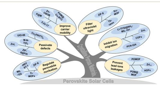
Fig. 18 Schematic illustration of application methods of various CPM and their functions in PSCs.
