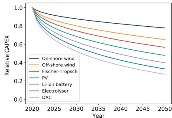
Fig. 7 CAPEX of the individual components of a jet fuel production plant,<sup>16,28,62,63,78–85,87–89,99</sup> normalised to their initial cost of 2020. PV and wind power costs in EUR per kWp, battery costs in EUR per kWh, electrolyser costs in EUR per kW<sub>el</sub>, Fischer–Tropsch synthesis plant costs in EUR per kW<sub>ch</sub>, DAC costs in EUR per (t<sub>CO<sub>2</sub></sub> a).
