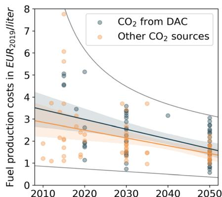
Fig. 3 Fuel production costs from literature review for CO<sub>2</sub> provision from DAC and other CO<sub>2</sub> sources. The depicted regression line of all 113 data points (with a 95% confidence interval shading) has an adjusted  $R^2$  value of 0.23 (0.13) for CO<sub>2</sub> from DAC (other sources), revealing the high spread in the data.
