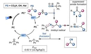
Scheme 2 Trityl isocyanide as a general reagent for photoredox catalyzed cyanation.
