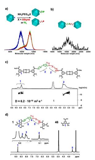
**Fig. 2** (a) Comparison of the MALDI-TOF spectra of (COOH)<sub>1</sub>-RhMOP (blue),  $(N_3)_1$ -RhMOP (green) and (alkyne)<sub>1</sub>-RhMOP (red) which evidences an increase in mass due to the attachment of a chain of NH<sub>2</sub>PEG<sub>38</sub>X to the MOP (where X = N<sub>3</sub> or alkyne). (b) MALDI-TOF spectrum of the MOP-dimer, showing the single broad peak centered at 18 538 m/z. (c) DOSY-NMR spectrum of the MOP-dimer. (d) <sup>1</sup>H-NMR spectrum of the acid-digested MOP-dimer.
