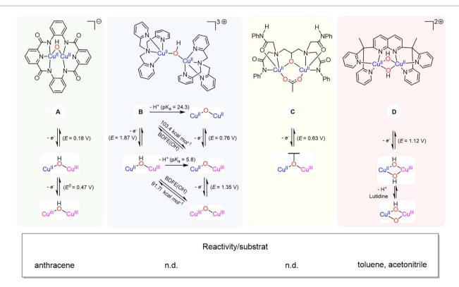
Fig. 9 (Top) Starting materials for the preparation of reported dicopper high valent species. (Down) Selected experimental properties (A (wet DMF),  $^{209}$  B $^{215}$  and D $^{216}$  (CH $_3$ CN) and C $^{210}$  (DMF)), E in V vs. Fc $^+$ /Fc.
