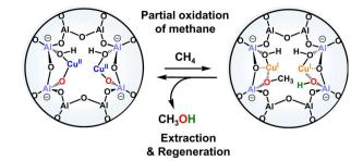
Fig. 20 Strategy used to generate monomeric  $[Cu]^{2+}$  sites in a pure alumina environment and the subsequent reaction with  $CH_4$  to form hydroxyl and methoxy species.
