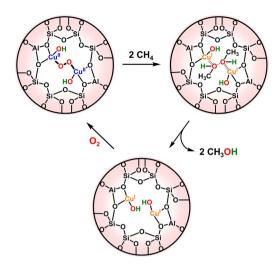
Fig. 18 Proposed catalytic cycle for the CH<sub>4</sub>/O<sub>2</sub>/H<sub>2</sub>O reaction over Cu zeolites.
