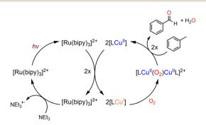
Scheme 12 Complex LCu(i) (L = tmpa (tris(2-pyridylmethyl)amine)) after reaction with O2 according Göttlich and Schindler206 and proposed general catalytic cycle for toluene oxidation (adapted from ref. 206).
