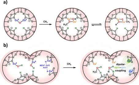
Fig. 14 Suggested reaction pathways of Cu-O species in Cu-MOR and their transformations during the reaction with CH<sub>4</sub>. (a) Pathway involving  $[Cu_2(\mu-O)]^{2+}$  species. (b) Pathway involving  $[CuOH]^+$  species, highlighting the inactivity of monomeric Cu species exhibiting dipolar spin-spin coupling at a separation distance of 4.8 Å.
